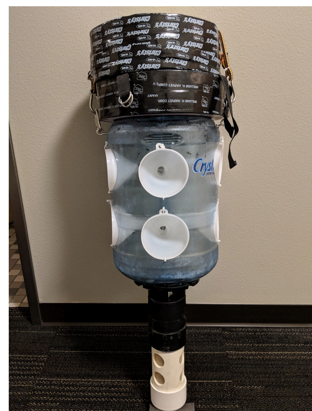
Figure 2: Dungeness crab trap. Top section includes the sensor control unit housed in an enclosing float. Middle section houses LED light and funnels for crab.
